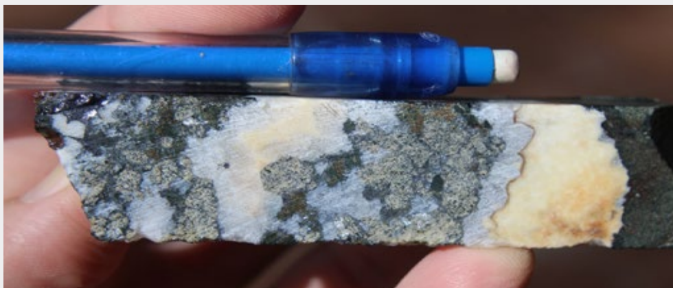
Figure 9: Drill core 1-0-5D - White sphalerite, quartz-carbonate vein in conglomerate at 13.5m depth
